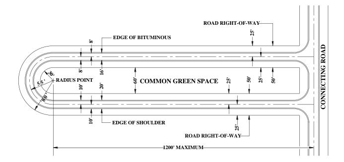
c. As an alternative to the rural design and construction standards, urban design (curbed) roads may be used if designed and constructed in accordance with the "Wisconsin Department of Transportation Standard Specifications for Highway and Structure Construction", the "Facilities Development Manual of the Wisconsin Department of Transportation" and the standards in the following table:
